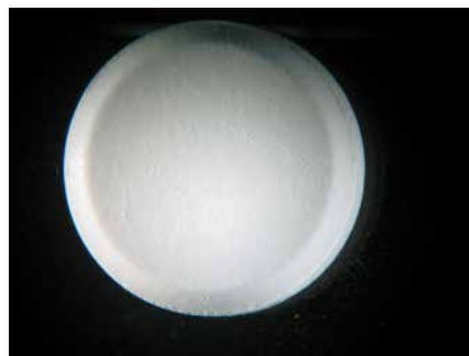
Figure 1. Parateck® Mg DC tablet with Starch 1500®, sample 1, compaction force 20 kN, Ø 11 mm, flat, faceted
